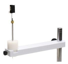
**Step 1:** Begin by inserting a guide tube into one of the small unthreaded holes in the guide body where the probe will be positioned. Slide the guide tube in until the bottom of the tube is flush with the bottom of the guide body.
